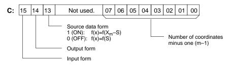
Enter the coordinates of the m+1 end-points, which define the m line segments, as shown in the following table. Enter all coordinates in BIN form. Always enter the coordinates from the lowest X value  $(X_1)$  to the highest  $(X_m)$ .  $X_0$  is 0000, and does not have to be entered.
